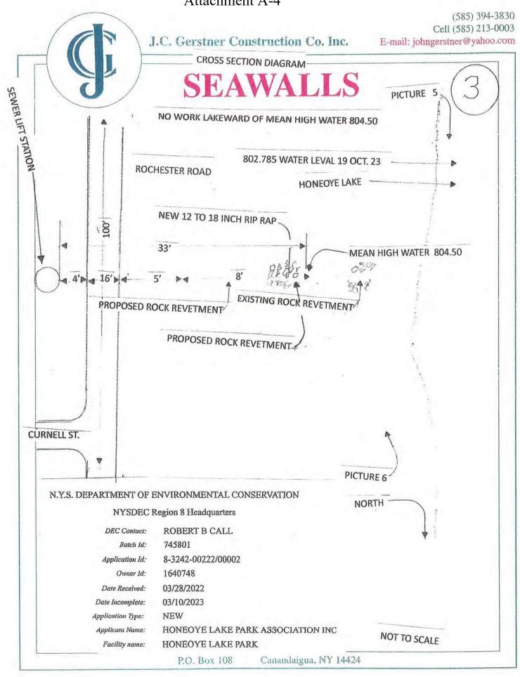
8-3242-00222/00002 Attachment A-5 (585) 394-3830 Cell (585) 213-0003 J.C. Gerstner Construction Co. Inc. E-mail: johngerstner@yahoo.com CROSS SECTION DIAGRAM PICTURE 5 NO WORK LAKEWARD OF MEAN HIGH WATER 804.50 802.785 WATER LEVAL 19 OCT. 23 ROCHESTER ROAD HONEOYE LAKE NEW 12 TO 18 INCH RIP RAP 33' MEAN HIGH WATER 804.50 050 EXISTING ROCK REVETMENT PROPOSED ROCK REVETMENT PROPOSED ROCK REVETMENT
